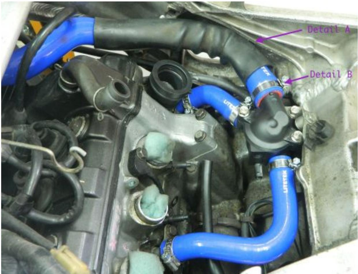
8. Fit the OEM protective PVC sleeve to protect the hose from chafing.
